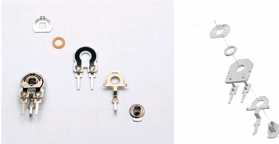
Figure 3: Example of a trimmer potentiometer (source: Tokyo Denshi)
