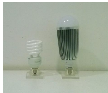
Figure 12: CFL 32W and LED 25W with same lumen package
