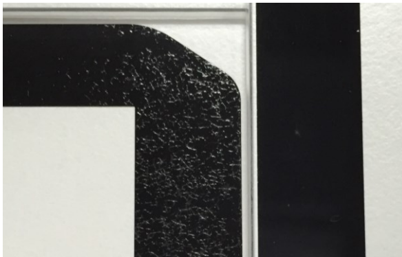
Picture 2: comparison of lead-free (left) and lead-containing (right) ink. On the left side the ink shows a so called “chipping”, i.e. peeling off from the substrate (borosilicate glass).
