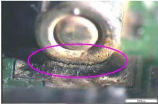
Solder joint is torn from the component
