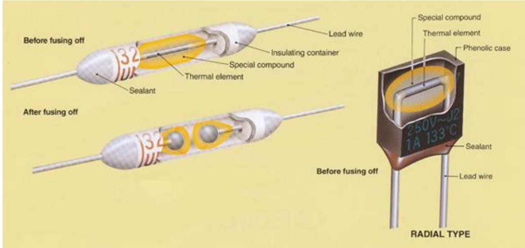
Eutectic alloy solder that connects to two electrical leads in a ceramic tube with epoxy sealed ends. This construction relies on the eutectic melting properties of certain metallic alloys. When the alloy melts it disconnects the conductive path between the lead wires. The temperature of the fusing is dictated by the choice of the appropriate alloy.
