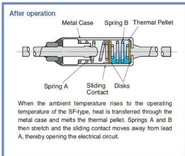
An organic thermal pellet holds a spring loaded sliding contact in place to create an electrical connection between the leads of the device. At the desired operating temperature, the thermal pellet melts thus allowing the sliding contact to move and open the connection between the leads of the device.
