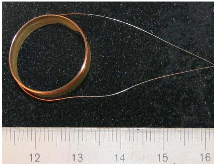
Figure 2: A voice-coil with a pre-tinned enamelled CCAW
