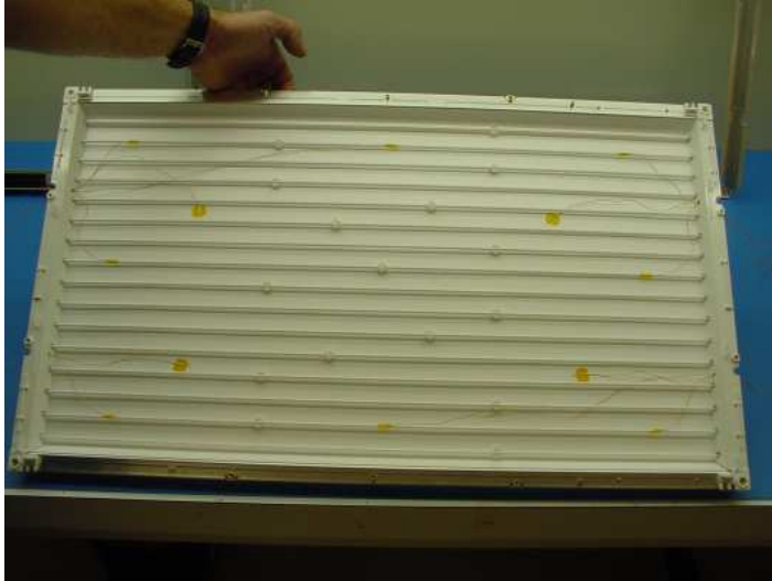
Figure 13. A partially disassembled LCD backlight (showing fluorescent lamps)
