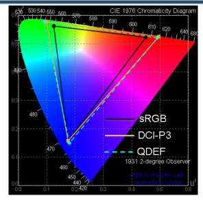
QDEFs with narrow green and red line-widths (~32nm) are necessary to achieve >98% DCI-P3 color-space coverage with current CF70 color filters
