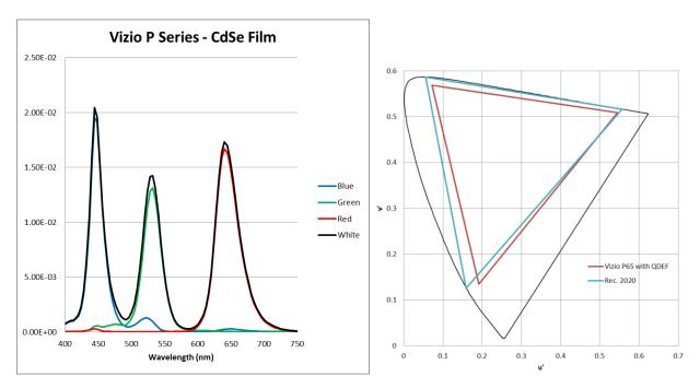
This set has a native white point of 7589K and Rec2020 (BT2020) color gamut coverage of 85.4% and also achieves 94% of the DCI-P3 specification and would therefore meet the color gamut requirements to be a UHDA compliant set. At the same time, the set has output brightness comparable to the YAG set (400 nits vs 450nits.)
