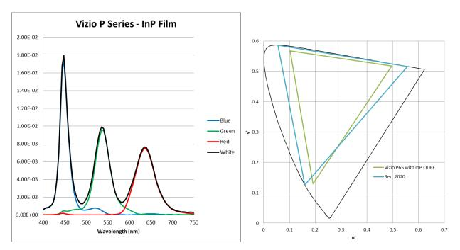
This set has a native white point of 6597K and Rec2020 (BT2020) color gamut coverage of 73.7%. This set does achieve 92.7% of the DCI-P3 specification and would therefore meet the color gamut requirements to be a UHDA compliant set, but overall brightness using the same input power is severely impacted. With only 350 nits out, this set can be seen have 23% less front of screen brightness than the YAG LED based set.
