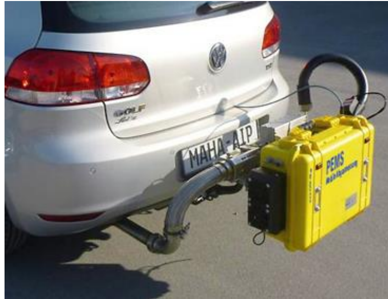
Image 4: Mobile test equipment based on InP quantum cascade laser
