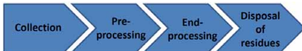
Figure 5-2: Generic recycling chain for end-of-life EEE
