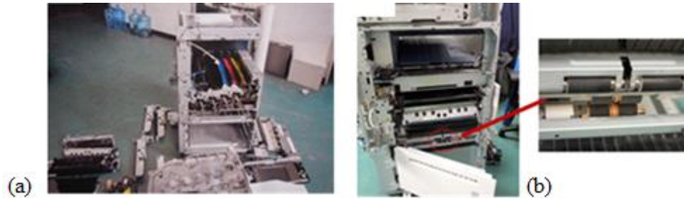
Figure 3.7 a) The disassembled individual parts of copier. b) One of the sensitive components in copiers.
