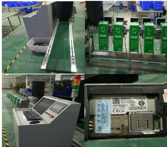
Figure 4.4 Identification machine for type of product and model reading the QR code
