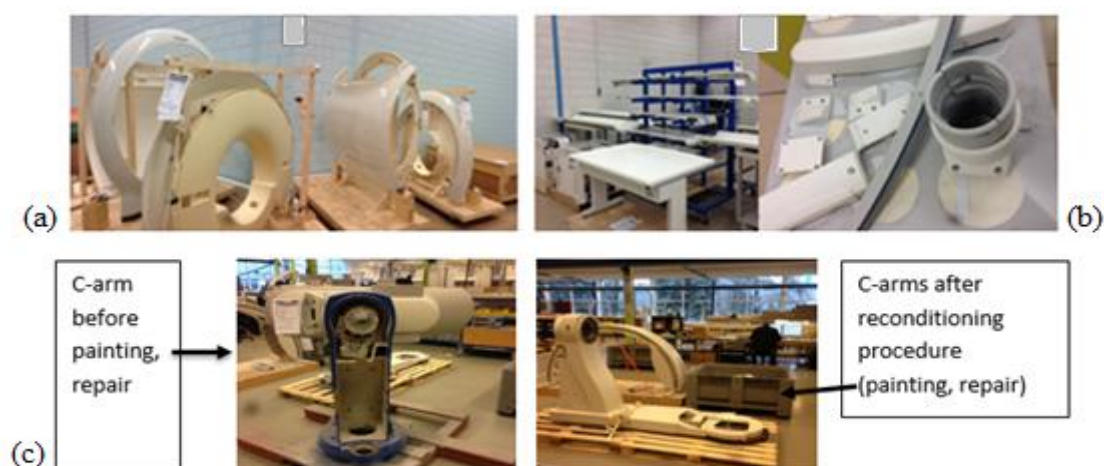
Figure 5.12 Body parts after repainting; a) MRI cover; b) Patient table components c) C-arm reconditioned
