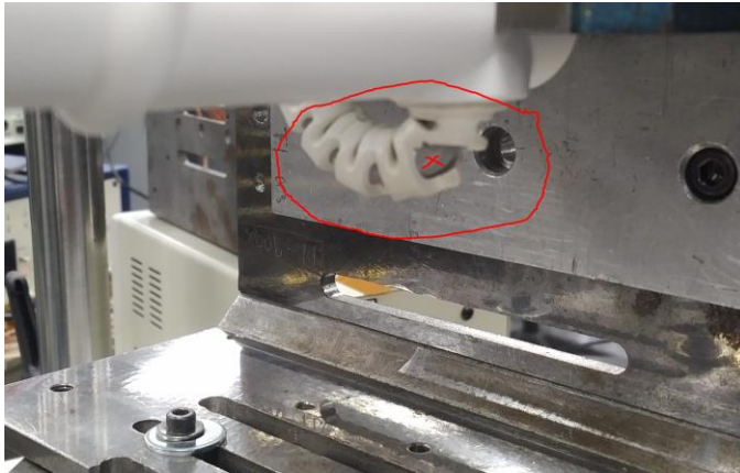
Figure 3. Cracked Bending Cycle
