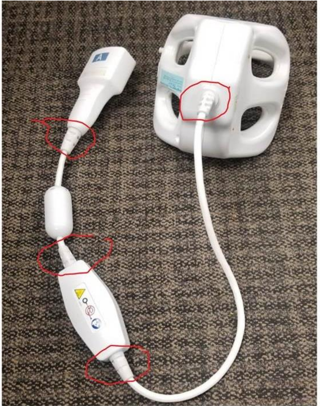
Figure 1. MRI coil for imaging shoulders. These connect to the MRI via the four strain relief boots shown above (circled in red).
