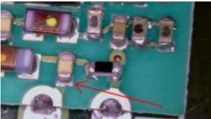
Figure 6: Lead-free soldered printed circuit board of an MRI with poor wetting at arrowed chip capacitor and other components (COCIR 2011)
