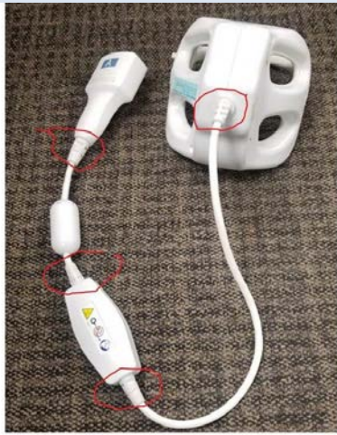
Figure 5-2: MRI coil for shoulder; the four strain relief boots are circled in red.
