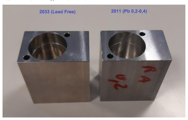
On the next page we indicate the measured roughness on the centre large hole of both samples.
