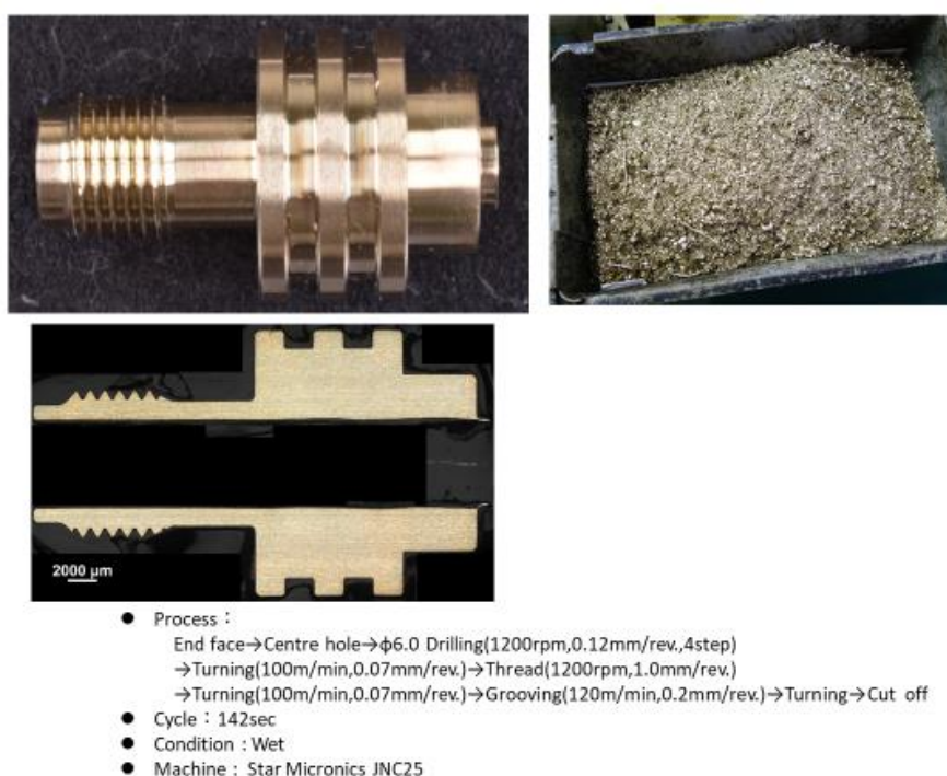
Fig. 10-1: Machining Example of Valve Part 4-1
