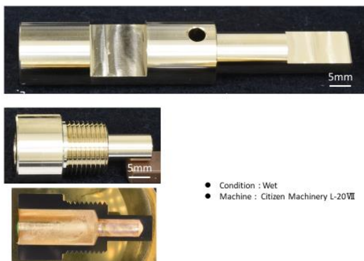
Fig. 25: Machining Example 9 –Component Requiring Milling and Component Similar to Temperature Sensor
