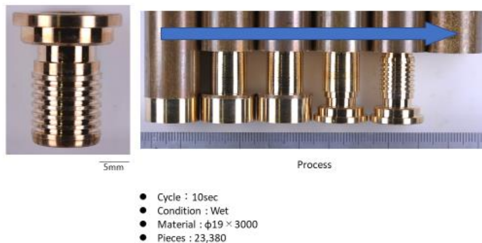
Fig. 8: Machining Example 2 – Machining with Automatic 6-Spindle Lathe
