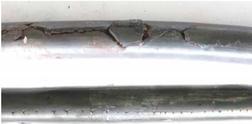
Figure 18-1: Cracks in bismuth containing steel wire rods after rolling
