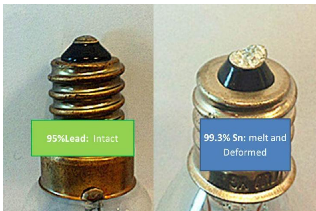
Figure 34-4: Oven lamp failure
