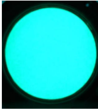
Figure 10: Typical MCP gain uniformity. There is no visible fixed pattern noise in the image.
