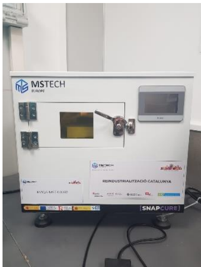
Figure 2.- Proprietary, fully functional MULTISMART UV LED curing oven developed by MSTECH.
