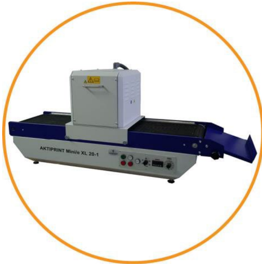
Belt dryer, continuous table-top device for rapid curing of UV Hg inks, UV coatings and UV adhesives in the small-format printing sector for testing or production on flat material and moulded parts, Example of size: (L×H×W) 105 x 40 x 50 cm, appr. 45 kg
