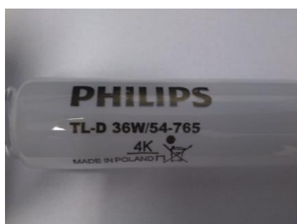
Good marking with Pb containing ink
