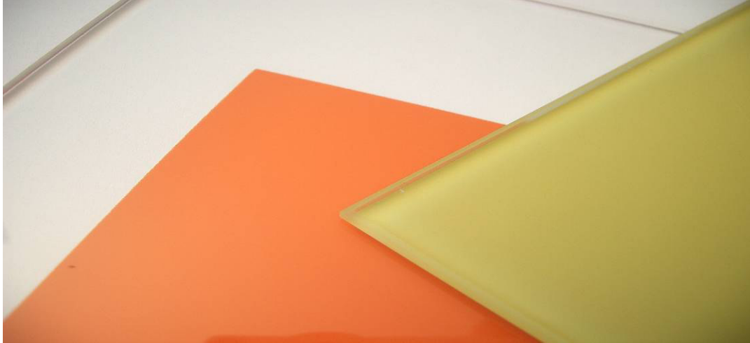
Picture 3: Enamels on glass giving bright orange (left) or yellow (right) colorings.
