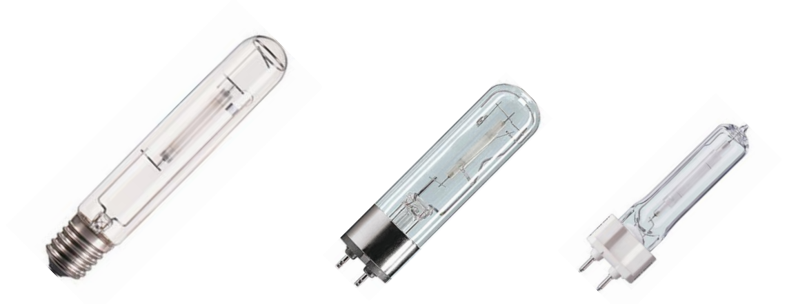
Figure 2: Different formats of High Pressure Sodium lamps with increased colour rendering: Edison cap, PG-12 and G12
