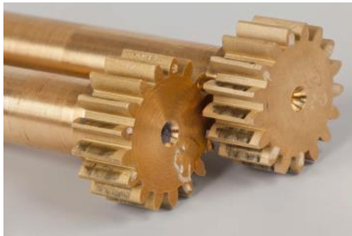
Picture 1: Gear pinions made from leaded brass CuZn39Pb3 (left) and lead-free brass CuZn31Mn2Si1Al1 (right) after wear test in combination with gear wheels made from POM.
