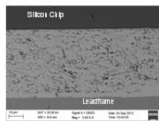
Cross-section of an adhesive with sintered silver particles (dark spots are remaining resin content).
