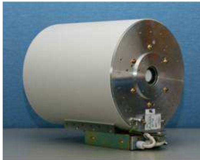
Figure 3. Fully assembled image intensifier which will be installed in the X-ray system
