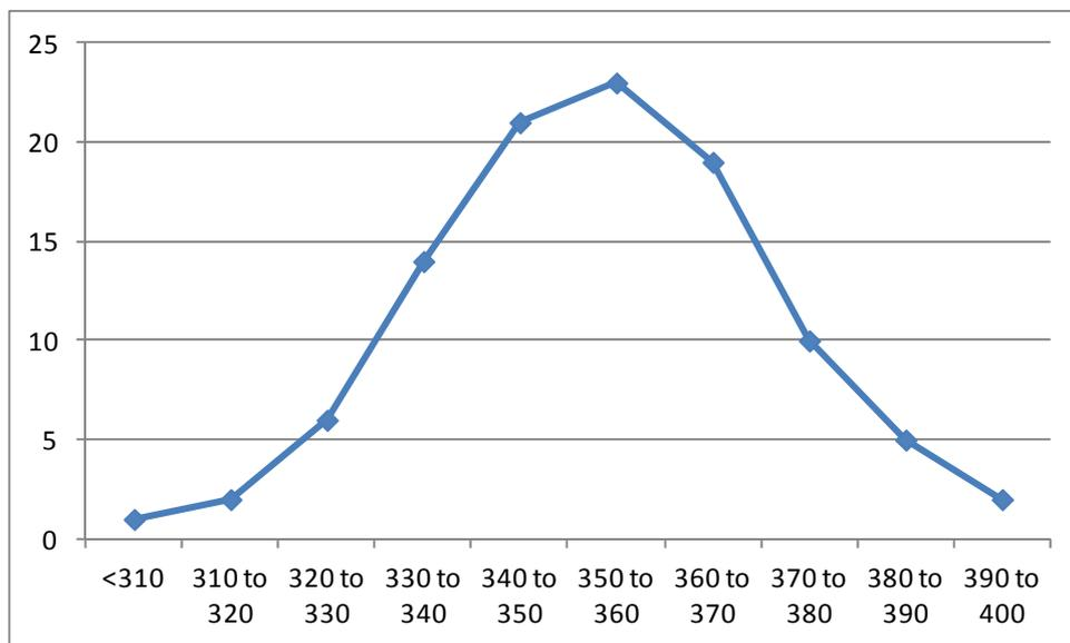
Figure 1. Required Spectral Distribution of Lamps used for Photoactivation of Methoxsalen
