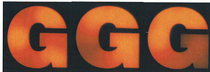
Figure 6. Reference conditions for each pattern: SPF1 (left), SPF2 (middle) and SPF3 (right). The contrast modulation value of these conditions was calculated at 0.70, 0.90 and 1.0, respectively.
