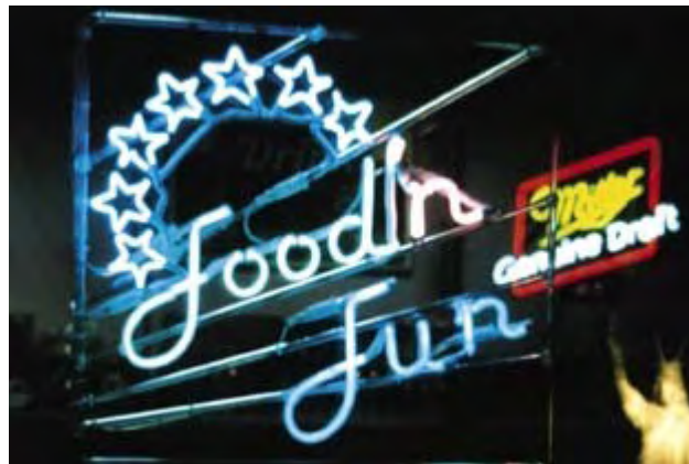
Fig. 2: A typical window neon sign. The series of stars was made from a single glass tube; the connecting parts, which are dark, were painted black after the glass fabrication.
