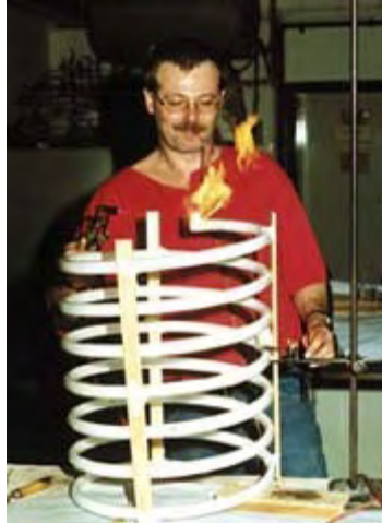
Fig. 3: A master neon glassblower attaches electrodes to a 25mm-diameter, cold-cathode tube spiral. The single tube's total length measures 27 ft.
