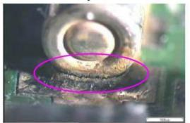
Solder joint is torn from the component
