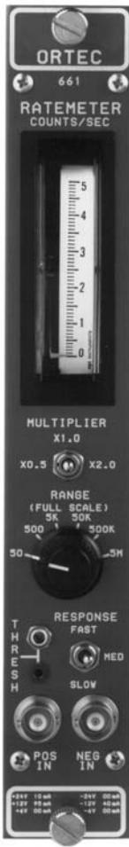
ORTEC Model 661 Ratemeter measures the counting rate of randomly arriving pulses, or the frequency of periodic signals in the range of 0 to  $10^7$  counts/s (0 to 10 MHz). This range of counting rates is covered with 18 different scales. The scales are arranged in a 25, 50, 100 sequence from 25 counts/s to  $10^7$  counts/s full scale.
