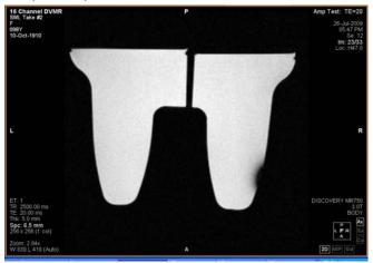
The image below demonstrates a loss of image on the upper left due to nickel on capacitor terminations.
