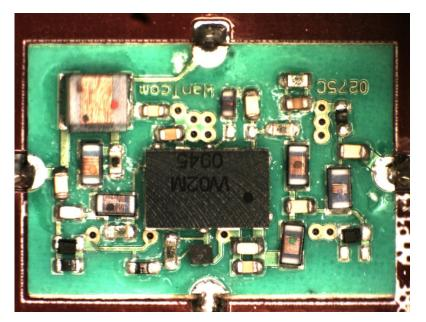
The above MRI PCB assembly is 10mm by 15mm (overall dimensions). Selectively soldering components of differing thermal mass is possible with relatively large leaded components but would be difficult with the small surface mount components and population densities employed in circuits such as the above pre-amplifier.
