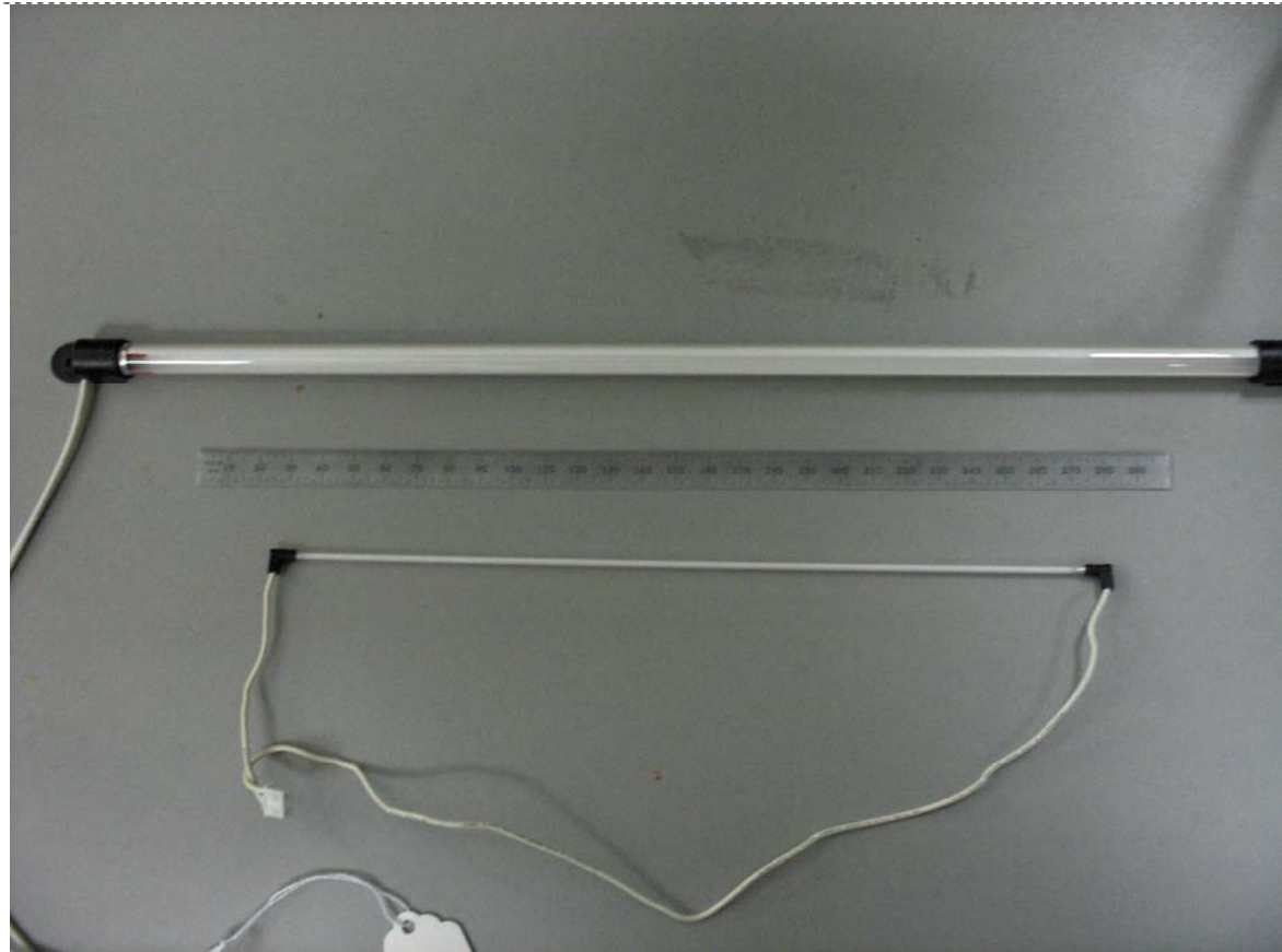
Xenon lamp on top, CCFL on bottom, scale is 300mm
